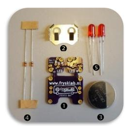
LED eyes can be soldered and tested in a manner of minutes. It can then be used, as-is, to add some bling to a craft project, or broken apart and sewed into a soft-circuit using conductive thread.
