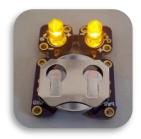
The **longer leg** on the Led indicates the positive, anode pin. (+) If someone trimmed the legs, try finding the flat edge on the LED's outer casing. The pin nearest the **flat edge of the LED** will be the negative, cathode pin. (-)
